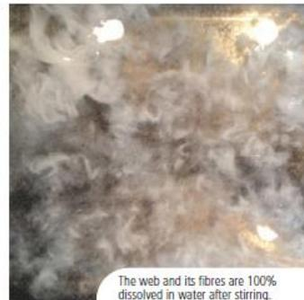
The web and its fibres are 100% dissolved in water after stirring.
